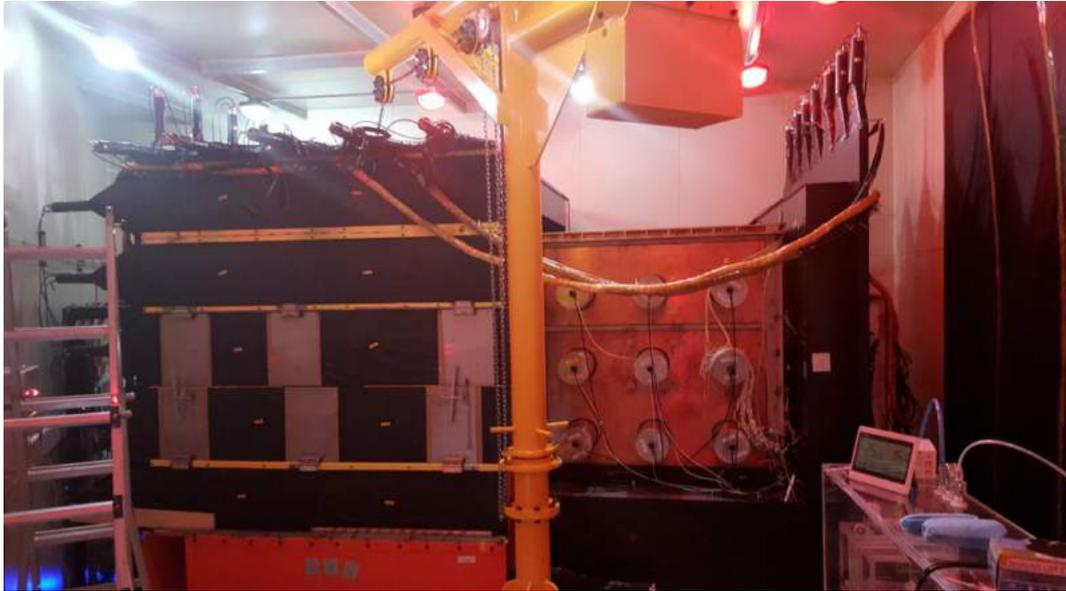
Figure III.3: A photo of the COSINE detector room when the front door was opened. Plastic scintillators with black covers and an orange copper box with 5" PMT assemblies on the A-side are shown. A hoist is used to move the 800 kg copper top.
