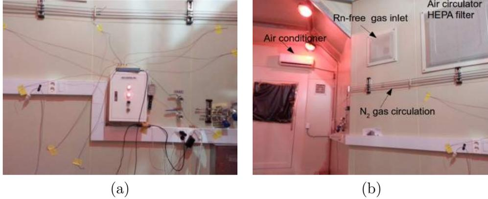
Figure III.14: (a) Test of temperature sensor thermocouples before installation. (b) Various environmental control system shown in COSINE-100.
